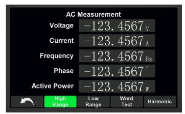
Click "Heavy current" or "Low range" to select corresponding gear while "Heavy current" can be used in direct perforation measurement, "Low range" can be used when accessing low current.
